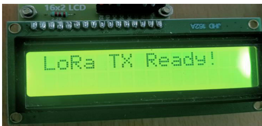
Figure. 5: LoRa transmitter initialization status display
